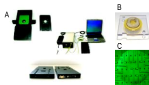
BioCell 100 set-up (A) for electrophysiological monitoring and a Multi-Electrode Array (M.E.A.) cartridge (B). In C an engineered neural tissue is positioned onto a M.E.A.
